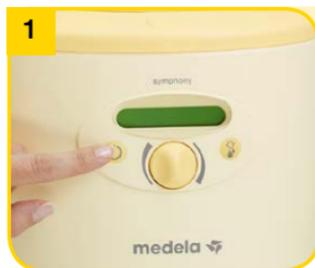
Press the On/Off button
