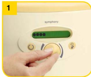
Set the comfort vacuum by rotating the vacuum adjustment knob. First rotate to the right to increase the vacuum until there is a slight discomfort. Then rotate to the left to reduce the vacuum until it is comfortable.
