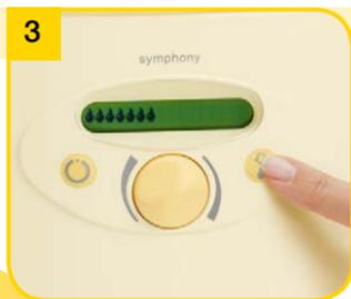
The pump will automatically switch to the expression phase after two minutes.
