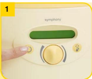
Press the On/off button
