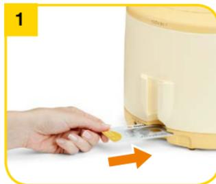
The program card must be inserted in the card compartment on the back of the breast pump. For more information on the use of the card and the selection of the appropriate program, see chapter 7.2.
