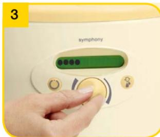
Set the comfort vacuum (see chapter 7.6). The bullets on the display show the vacuum level. The more bullets, the stronger the vacuum.
