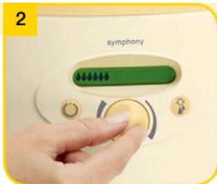
Set the comfort vacuum for the stimulation phase (see chapter 7.6). The drops on the display show the vacuum level. The more drops, the stronger the vacuum.
