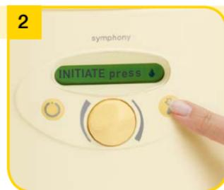
Press the "Let-down" button
