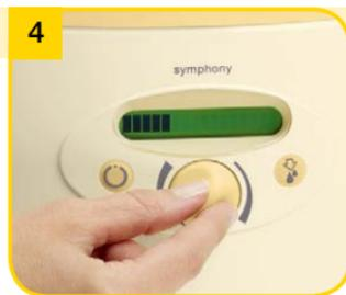
Set the comfort vacuum for the expression phase (see chapter 7.6). The bars on the display show the vacuum level. The more bars, the stronger the vacuum.
