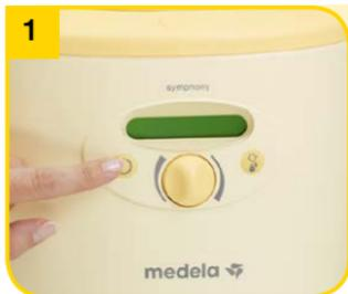
Press the On/off button
